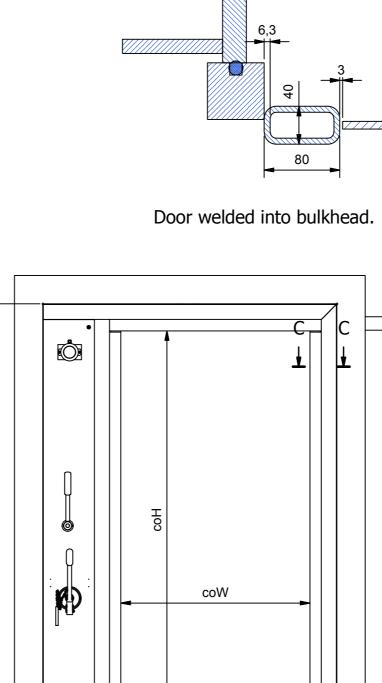
C-C Typical welding. —Bulkhead ship, no part of delivery 80
